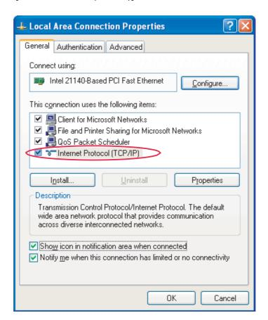
4-4 If the printer IP address is "192.168.1.253", enter any value from "192.168.1.1" to "192.168.1.252" or "192.168.1.254" in [IP address] field.
