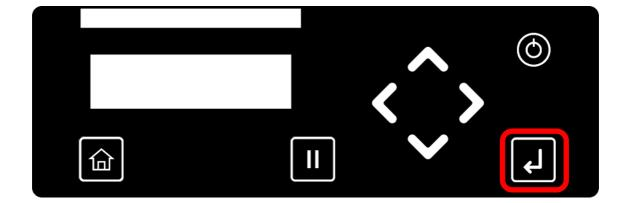
3. Use the [^] and [v] keys to change the value in the ranges "0-9 and A-F". Use the [>] and [<] keys to change the input position.
