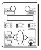
3. Use the [+] and [-] keys to change the value in the ranges "0-9 and A-F". Use the [>] and [<] keys to change the input position.
