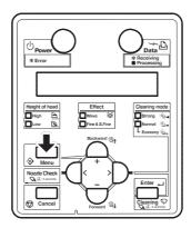
2-3 Use the [+] and [-] keys on the operation panel to display "Set \*\*: IP Address".
